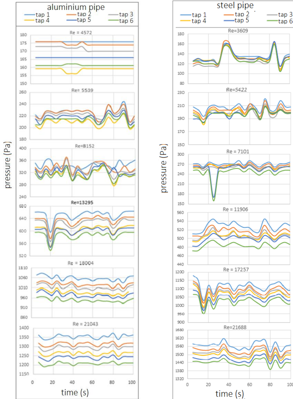
Figure 6. Time dependent variation of pressures at each taps location in different Reynolds numbers
