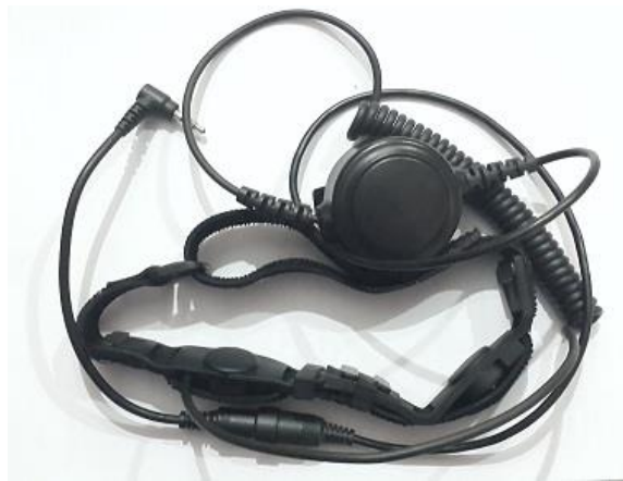
Figure 4. Throat microphone with two sensors
