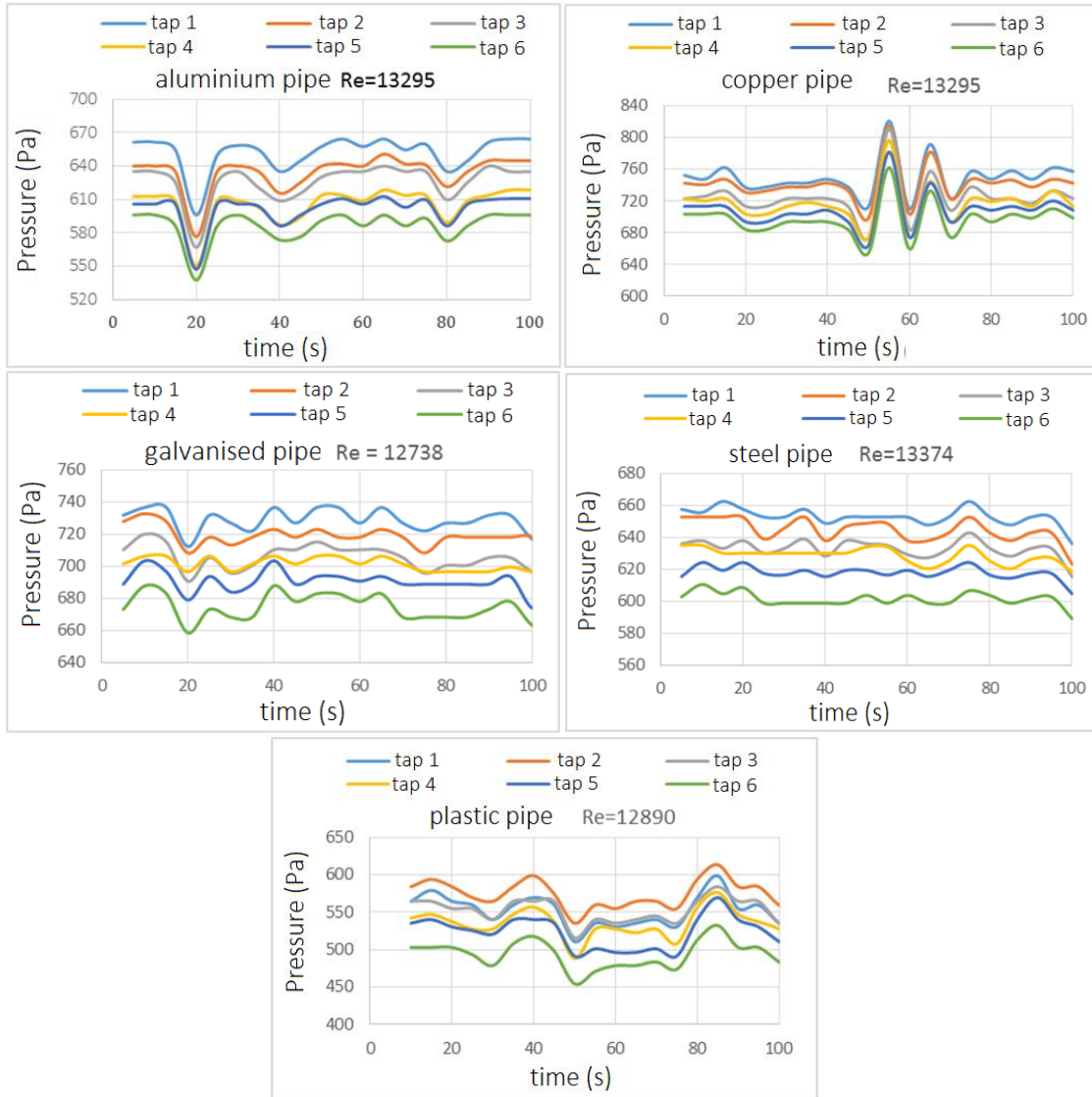
Figure 7. Variation of pressures across the time at each tap locations of five pipe type flows at close Reynolds numbers
